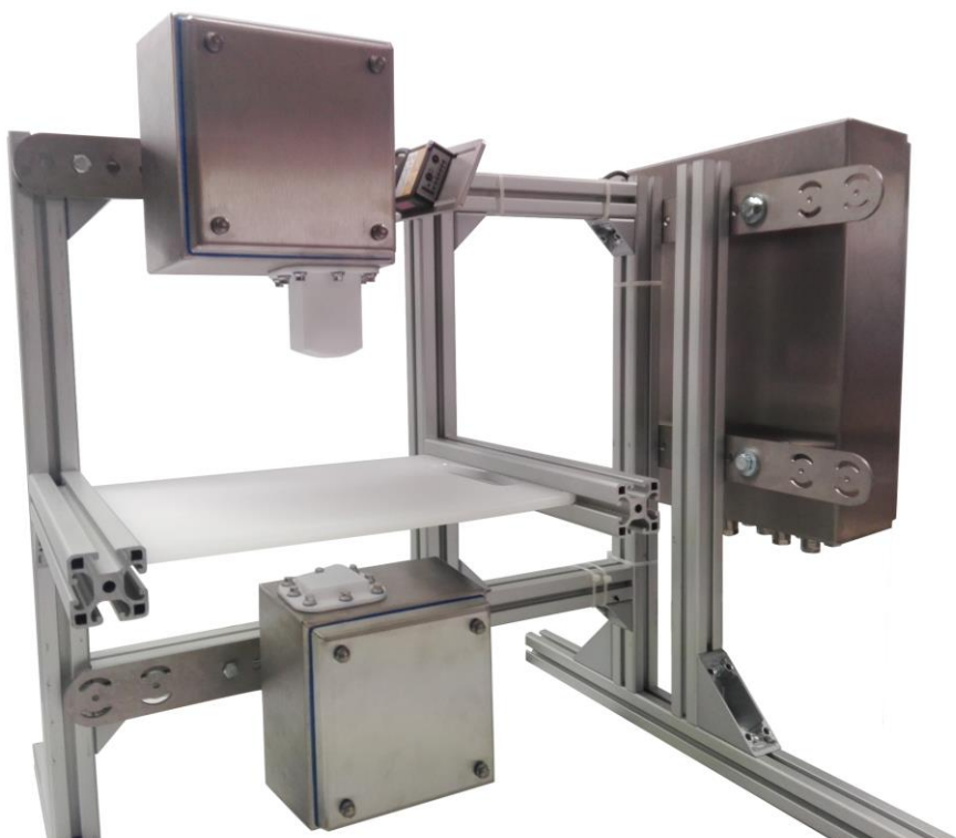
Figure 2: CALLIFREEZE® with emitter, receiver and computing unit.
